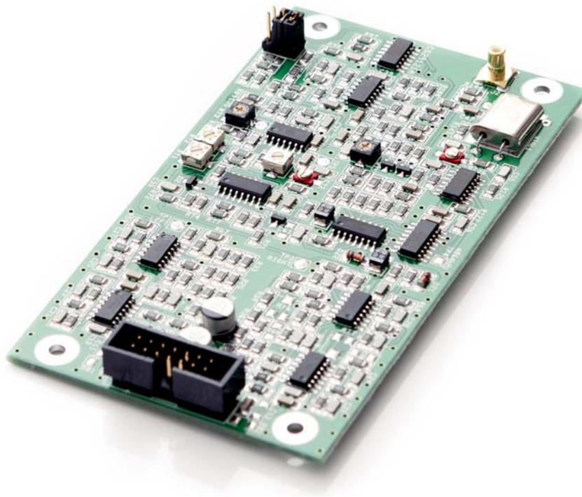
SEXC23COD2 board is a full fladged multiplex stereo encoder specially designed to be incorporated in SIELCO Transmitters. It incorporates the left and right 15kHz channel filters and the management of the monophonic transmission but not the pre-emphasis network which is managed by the transmitter. The card is easily installed in the factory or on the field on any SIELCO FM or STL Transmitter of the EXCxx5, EXCxxGT, EXC18 and EXC19 series.
